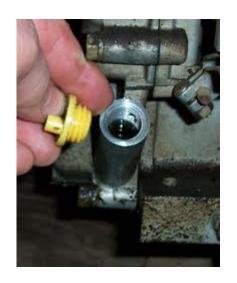
Drain oil, Change filter (if applicable) oiling Oring, refill, run engine for a minute, recheck level... easy...
