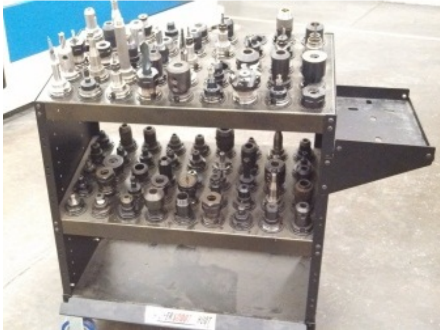
Figure 9: Illustration of an organized CNC tool cart with CAT40 Holders (Image by Ladell Humphries, 2013)
