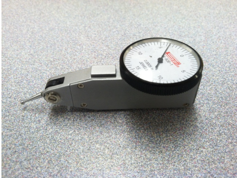
Figure 15: a Test Indicator in a horizontal view (Image by Machine Tool instructor: Ladell Humphries, 2013)
