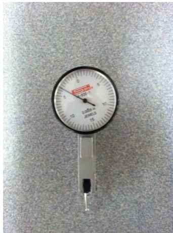
Figure 14: Test Indicator in a vertical view (Image by Machine Tool instructor: Ladell Humphries, 2013)
