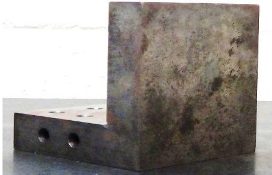
Figure 7: Images of an Angle Plate (Image by Ladell Humphries, 2013)
