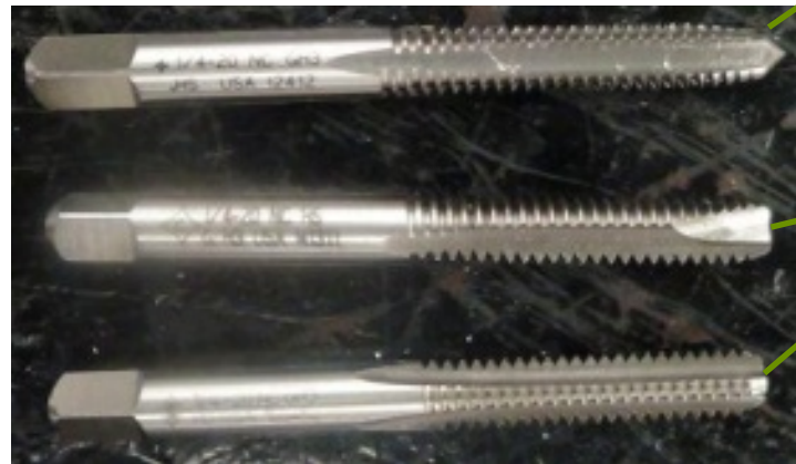
Figure 5: Types of Chamfers found on common taps (Image by Eddie Humphries, 2013)
