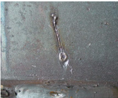
Example of an Arc Strike
