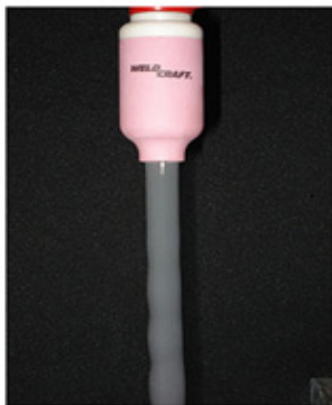
This photo shows the even gas flow created by using a gas lens.
