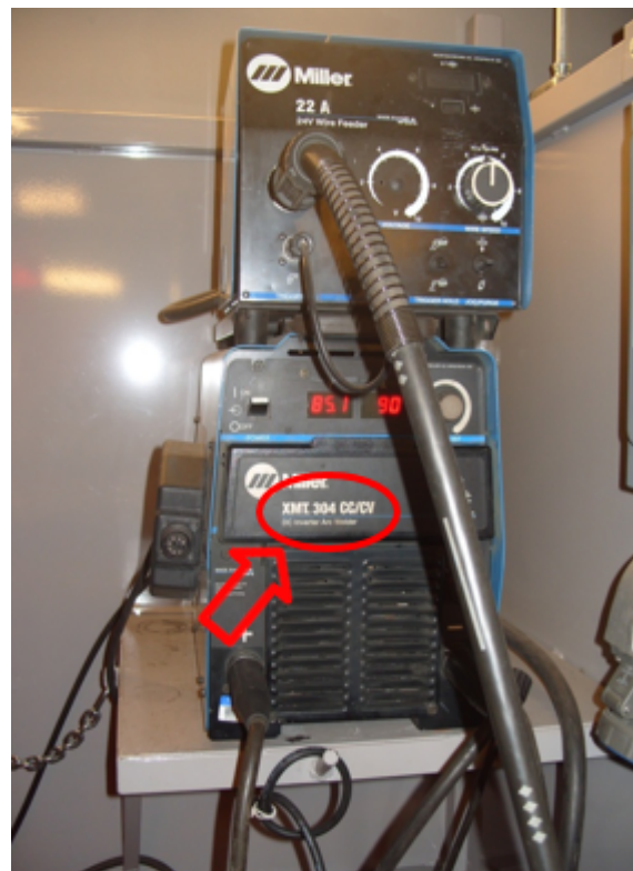
Figure 21. SMAW Machine with CC and CV Capability (by Paul Phelps, CC BY 4.0)
