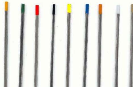
Figure 34. Image of Tungsten Electrodes with Color Bands (by Unknown, Public Domain)
