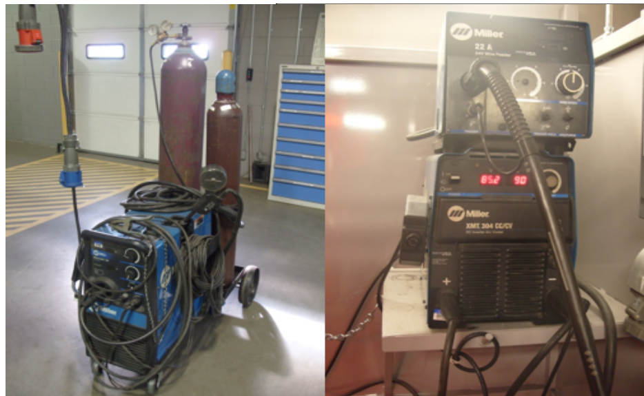
Figure 28. Examples of GMAW Set Ups (by Paul Phelps, CC BY 4.0)
