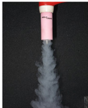
Photo shows gas coverage without a gas lens.
