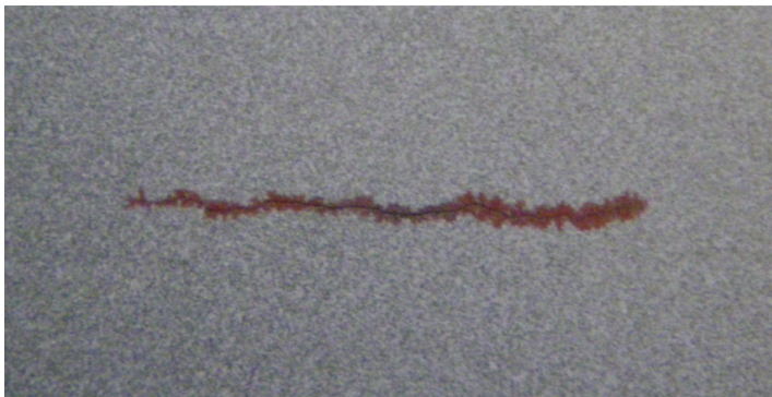
Figure 25. Results of Dye Penetrant Test (by Unknown, Public Domain)
