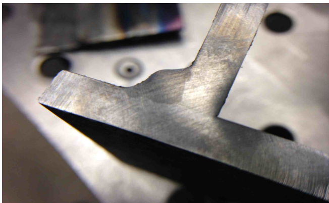
Figure 21. Macro Etch Test Weld (by Unknown, Public Domain)
