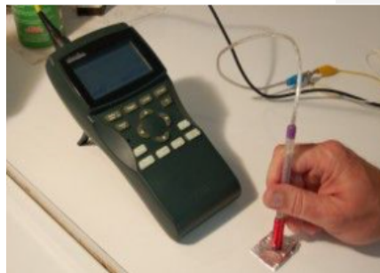
Figure 35. Eddy Current Testing on a Piece of Aluminum (by Jason Church, Public Domain)
