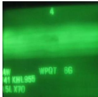
Figure 29. Weld Radiograph with Burn through Defect (by Bernoullies, CC BY-SA 3.0)
