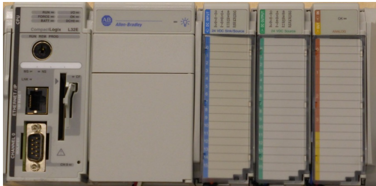
Modular I/O system Mounted on a DIN rail
