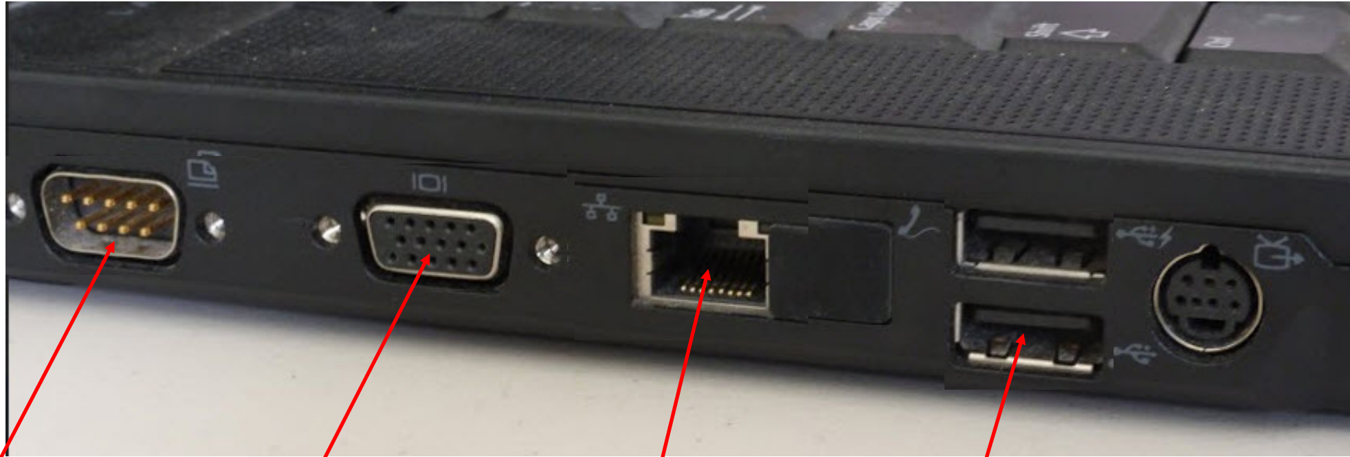
RS-232 port, which is a 9-pin, D shell connector
