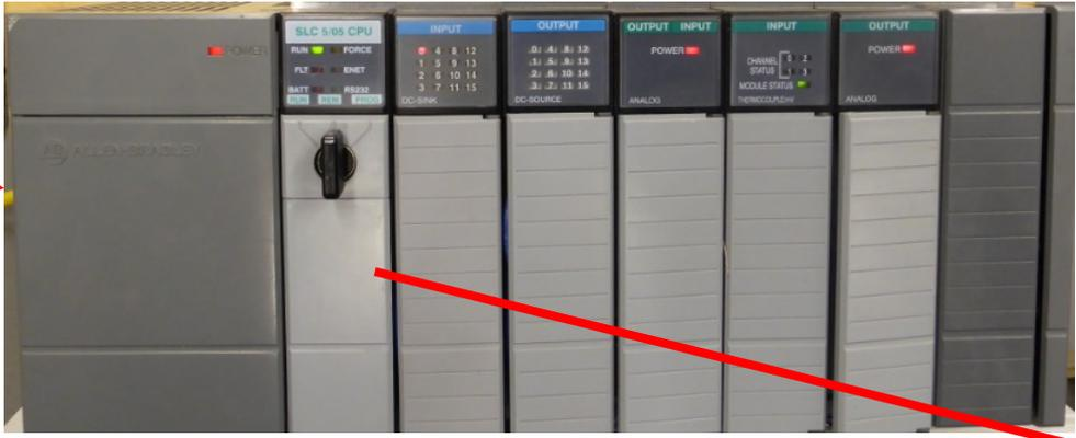
SLC-500 chassis, power supply, processor & I/O modules
