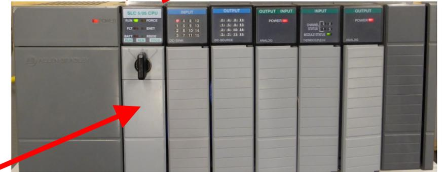
When the PLC project is downloaded, the processor must be in program mode, thus the machine will be shut down. You cannot download to a processor that is in run mode
