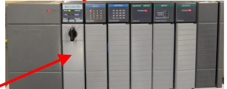
When the PLC project is uploaded, the processor can be in either the Run or Program mode. If the user is Online, click the save icon and it will do an Upload.
