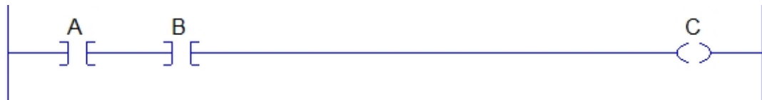
Figure 5A. AND Rung Logic.
