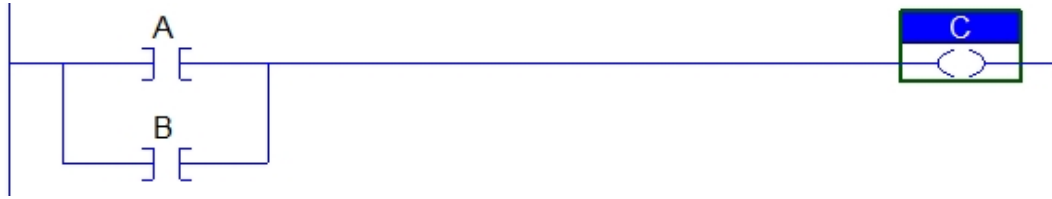
Figure 6-A. OR Rung logic.
