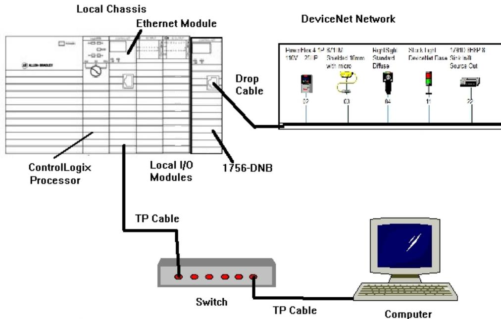
Figure 1-A. The hardware configuration for this HOA.
