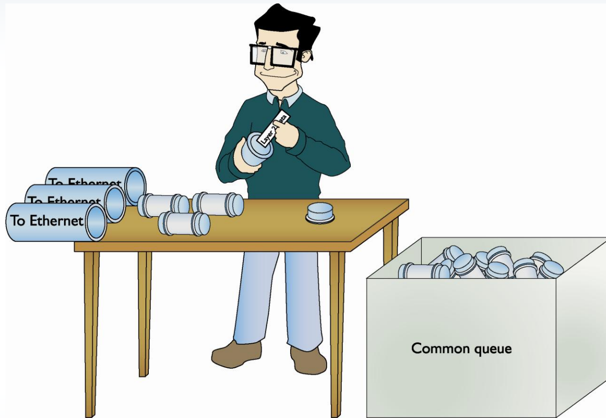
Figure 8.6 All incoming packets stripped of Layer 2 data and dropped into a common queue
