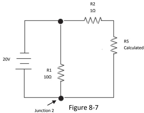
12. Look at the complex circuit identified in Figure 8-7. Because it is still a complex circuit you will need to break it down into pieces in which you can manage. Begin by visualizing how Figure 8-7 could be reduced to an equivalent circuit containing two parallel resistors.
