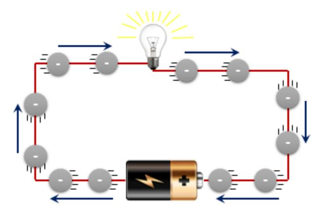
Direction of Electron Flow in a Simple Circuit
