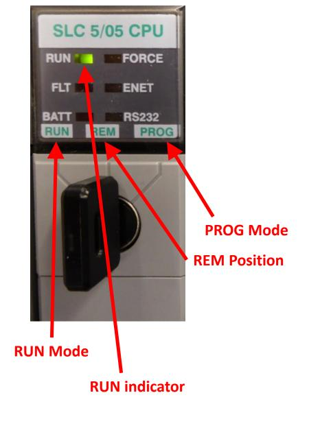
When the key-switch on the processor is in the **RUN position**, the processor is in the RUN mode. The RUN indicator will be on. In this mode the outputs will be enabled, thus the ladder program will control the outputs.
