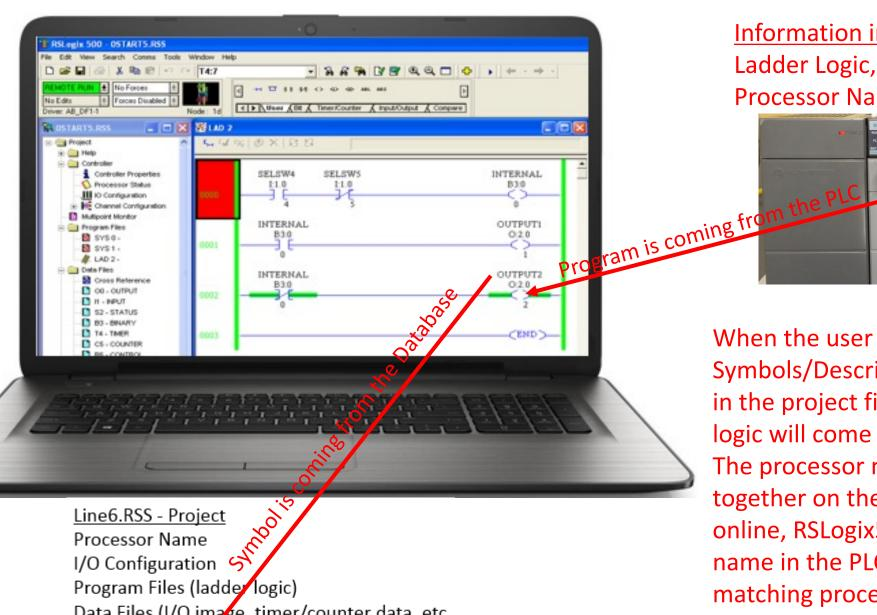
Information in Processor after Download Ladder Logic, Data Files Processor Name, I/O Configuration
