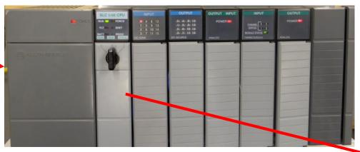
SLC-500 chassis, power supply, processor & I/O modules
