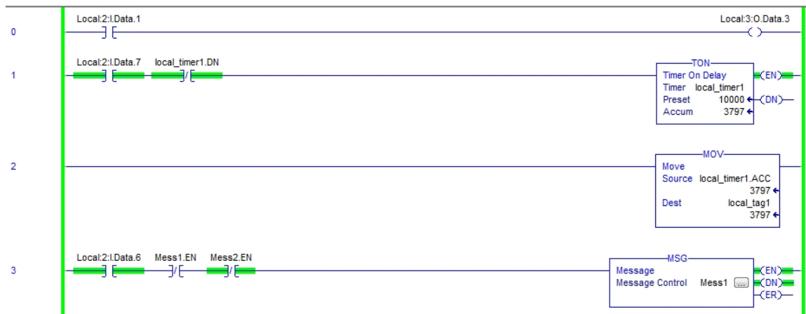
Figure 32-A Ladder Logic - Source Chassis
