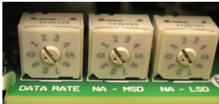
Figure 2-A Rotary Switches – Manual Setup
