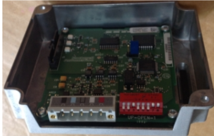
Figure 2-A 22-COMM-D DeviceNet Adapter in 22-XCOMM-DC –Base
